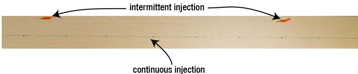
Improved dispersion through continuous injection best assures that the closest to ideal injection rate can be used to fully treat the flow stream. In real world applications, operators have reported significant performance gains after retrofitting from an intermittent to a continuous pump:
