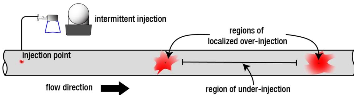
Most chemical pumps today are controlled by a timer to achieve a given number chemical doses per minute. For example, a pump that outputs a maximum of 100 Q/d would run 10% of the time to output a desired value of 10 Q/d. The on/off timer would run the pump on for, say 1 second, and off for the next 9 seconds of a 10 second cycle.
